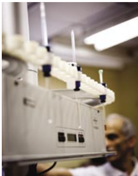
Faculty of Pharmacy & Pharmaceutical Sciences technician Vishwa Somayaji loading novel drug samples in thin glass vials in preparation for NMR-mass spectroscopic analysis of the newly synthesized products.
